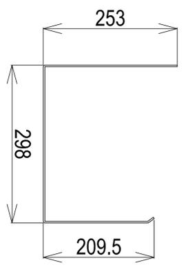
MEDIDAS DA CALHA PLUVIAL
